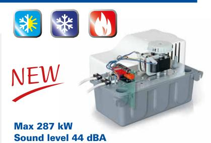
Pump for evacuation of condensate from boilers, the level of condensate inside the pump is managed without moving mechanical components, this provides great reliability. The functionality is guaranteed by software also with the presence of dirt. The new internal structure of the pump provides greater insulation from corrosive fumes and vapours from the tank. The NTH360 DIGITAL pump can be powered with an independent system from the boiler maintaining the alarm intervention active. (FIG.1)
